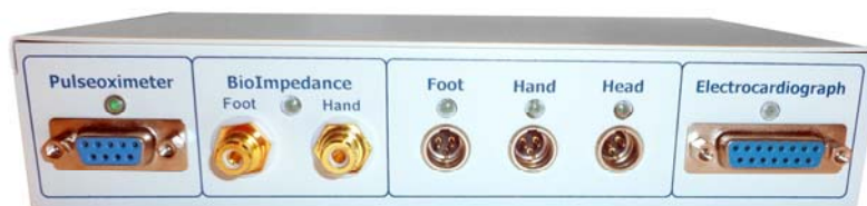
Fig. 1 Device Bioscanner Wellness . Bioscanner-04M embodiment. (Attention: the manufacturer has the right to change overall device dimensions without notice to customer).
